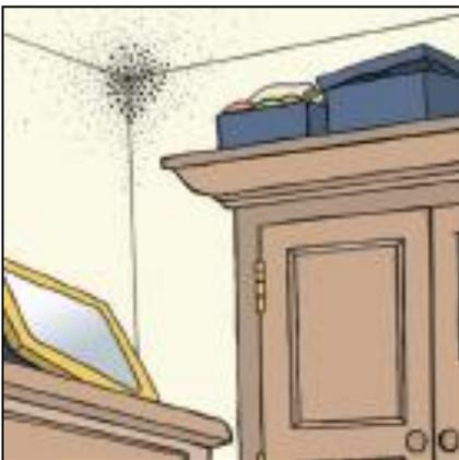
Condensation is caused by water vapour or moisture from inside the dwelling coming into contact with a colder surface, such as a window or a wall. The resultant water drops, the condensation, may then soak into the wallpaper, paintwork or even plasterwork. In time the affected damp area attracts black mould that grows on the surface.
